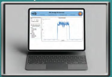
\* From the Daily Data screen, you can select and graph any of the dredges logged data for a given date. The last 60 days of data are available on this page to view.
